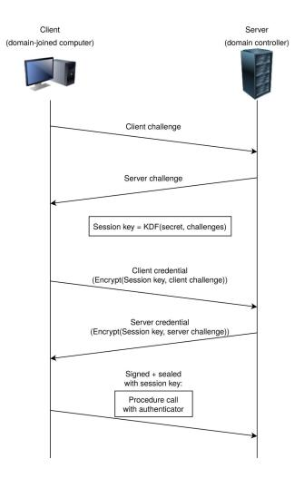
Figure 1: Simplified Netlogon authentication handshake
